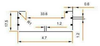
since profile is often employed for false ceiling and regarding the frequency of false celling implementation, F47 is one of the most widely used profile in drywall system.
